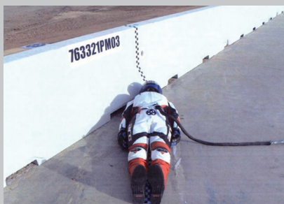
Picture 4 – Images from the full scale crash test on a rigid system: before, during and after the impact
